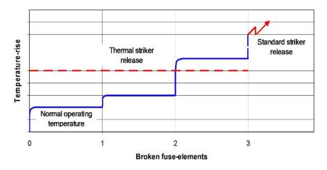
For all above reasons, use of thermal protection is highly recommended whenever fuses are used in combination with on-load switching devices.
